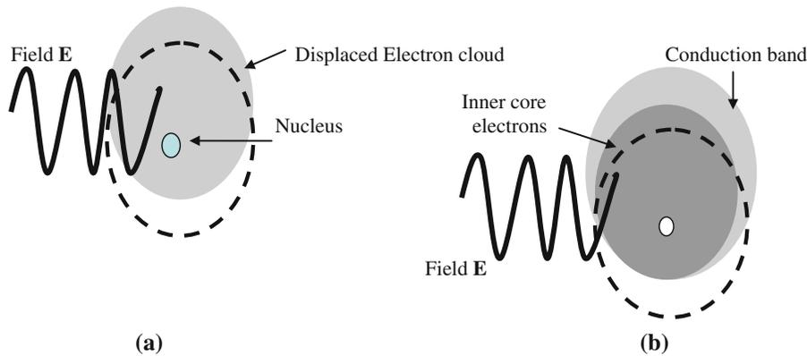
**Fig. 1** Interaction between the IB and CB electrons with electromagnetic field
